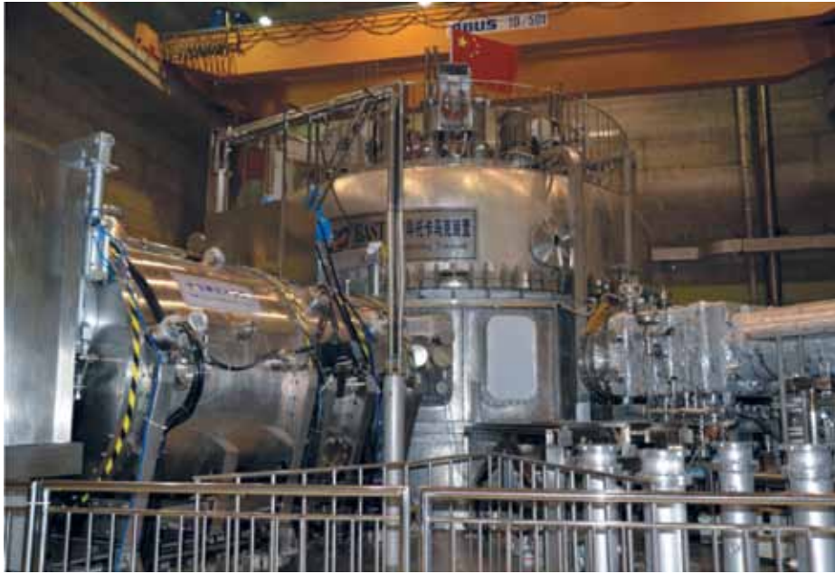
The Experimental Advanced Superconducting Tokamak at China's Institute of Plasma Physics, in Hefei.
