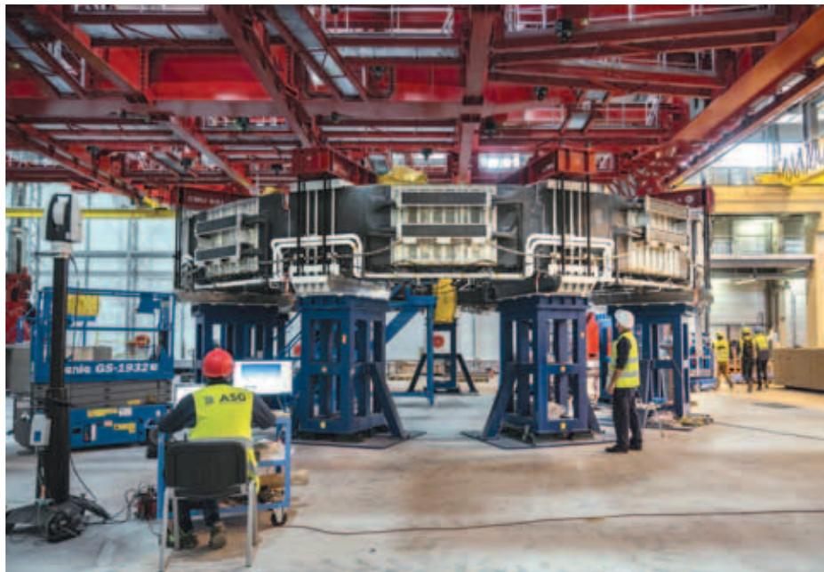
*ITER's 400-ton Poloidal Field Coil #6, fabricated in China.*
